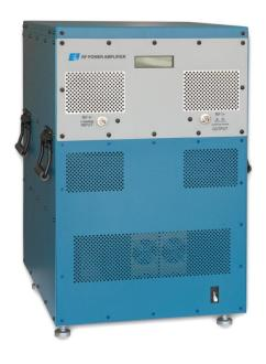
The 2500L Amplifier is a rugged source of RF power for ultrasonics, induction heating and laser modulation as well as plasma applications. It is a totally solid state solution employing RF DMoS FETs in the amplification power stages, offerina simultaneous forward and reverse power readouts, and an RS232 port for data 2500L reflects E&I's collection. The commitment to reliable and robust RF power.
