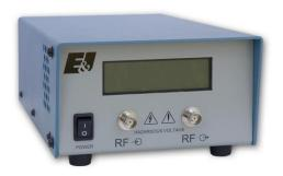
The PI-2 RF power indicator is used to measure the RF level of signal sources in the 10 KHz to 2 MHz range. Measuring RMS power to an accuracy of +/-3% over the entire frequency range, this portable unit is self-contained with an easy to read LCD display.
