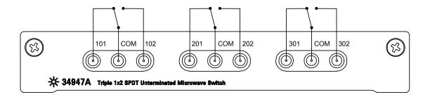
Figure 4 34947A Simplified Schematic
