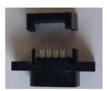
**4** Feed the ribbon cable up from the bottom. Ensure the cable is centered and straight (90 degrees to the edge of the connector), then gentle squeeze the connector to slightly pinch the cable and prevent it from moving.
