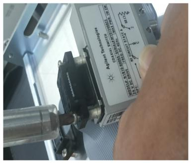
**2** Fasten the two screws (0515-1410) provided in the kit using 9 in-lbs torque with T10 torx bit to secure the switch to the chassis.
