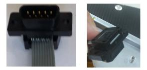
Inspect your completed cable. The ribbons should be snuggly clamped, and extend straight out from the connectors.
