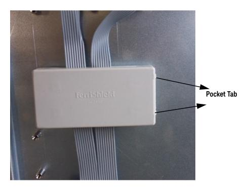
**2** Rotate top half onto bottom clipping both sides in one smooth motion.
