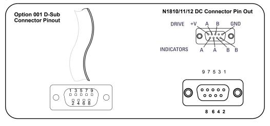
Figure 2 N1810/11/12 Switch and D-Sub Connector Pinouts
