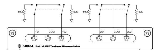
Figure 3 34946A Simplified Schematic
