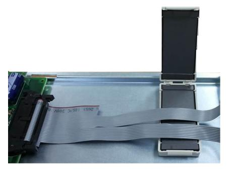
**3** Remove the ferrite suppressor.
