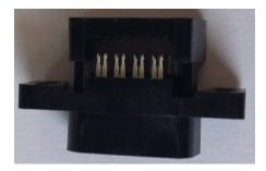
**3** Detach the 2 halves of the connector as shown below:
