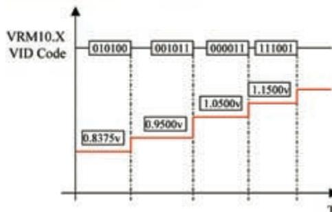
The 62000P Supplies provide 8 output TTL bits with timing control. These control lines can be used for VID control of VRM or to control other discrete signals.
