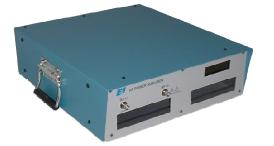
The 1040L Amplifier is a rugged source of RF power for ultrasonics, induction heating and laser modulation as well as plasma applications. It is a totally solid state solution employing RF DMoS FETs in the power amplification stages, offering simultaneous forward and reverse power readouts, and RS232 port for data collection. The 1040L reflects E&I's commitment to reliable and robust RF power.
