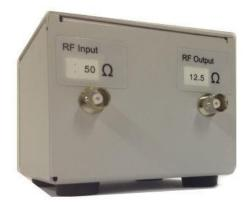
The JT-series of matching transformers allow you to transform the output impedance to match that of the amplifier; thus allowing you to increase peak-to-peak voltage without having to increase power. The transformers feature compact designs, allowing them to easily be placed in close proximity to the load and therefore minimize and losses due to the Q of your network.
