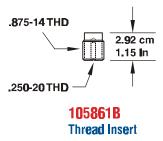
The bottom side of the antenna adaptor has a 7/8 in. by 14 threaded receptacle for mounting the adaptor on a tower or tripod, if this is not the desired receptacle size, thread the 1/4 in. by 20 thread insert into the adaptor. Take care not to cross thread this connection as permanent damage to the adaptor and insert could occur.
