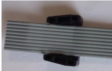
If you do this step wrong, your cable will be useless, so STOP and make sure you understand this step. You need to have the connectors oriented correctly on the cable. Ensure the cable is in straight.
