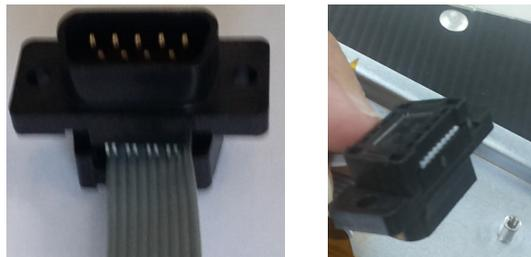
Inspect your completed cable. The ribbons should be snugly clamped, and extend straight out from the connectors.
