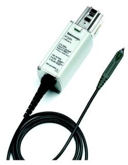
The P7225 probe offers a wide 8  $V_{\text{P-P}}$  dynamic range to access today's voltage levels with ultra-low input capacitance and high input resistance to take measurements with minimal signal distortion.
